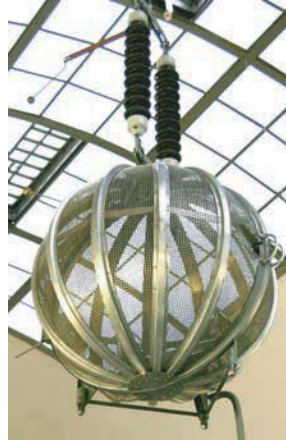
Faraday cage: to capture / shield energy pulses
